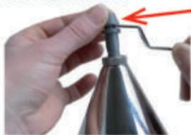
1. Insert the bar in the groove of the nozzle.
